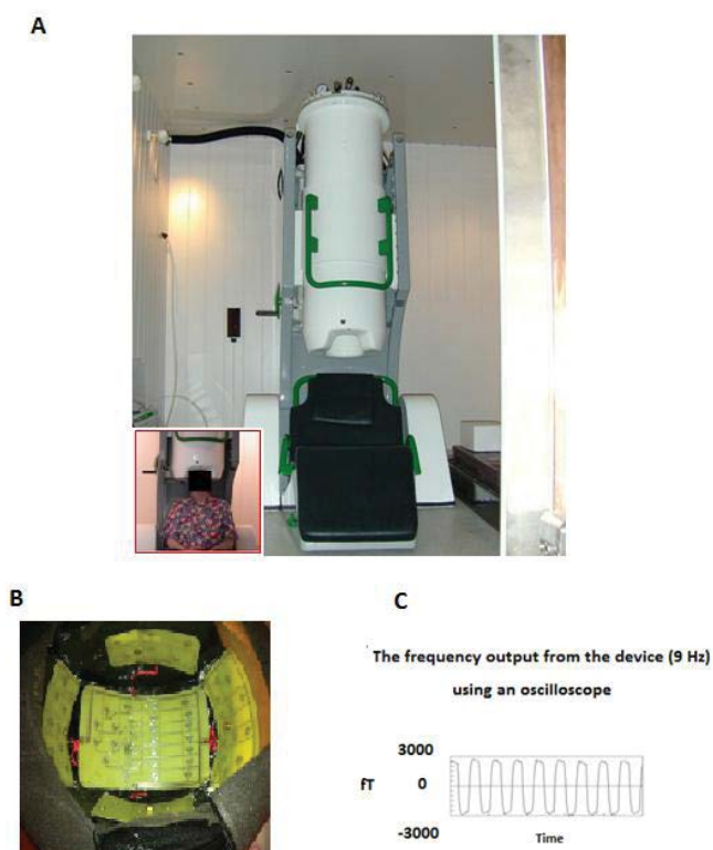
Figure 1: A) The 122 channel MEG system inside the shielded room and a patient during MEG recording (small photo). B) The configuration of the stimulation coils within the helmet of the electronic device. C) The frequency output from the electronic device which has calibrated to 9Hz.
